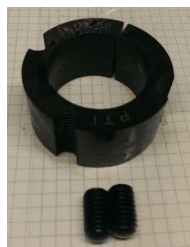
2000101610038 - Taperlock For vertical Ø38 5,5 and 7,5 Kw. motor
