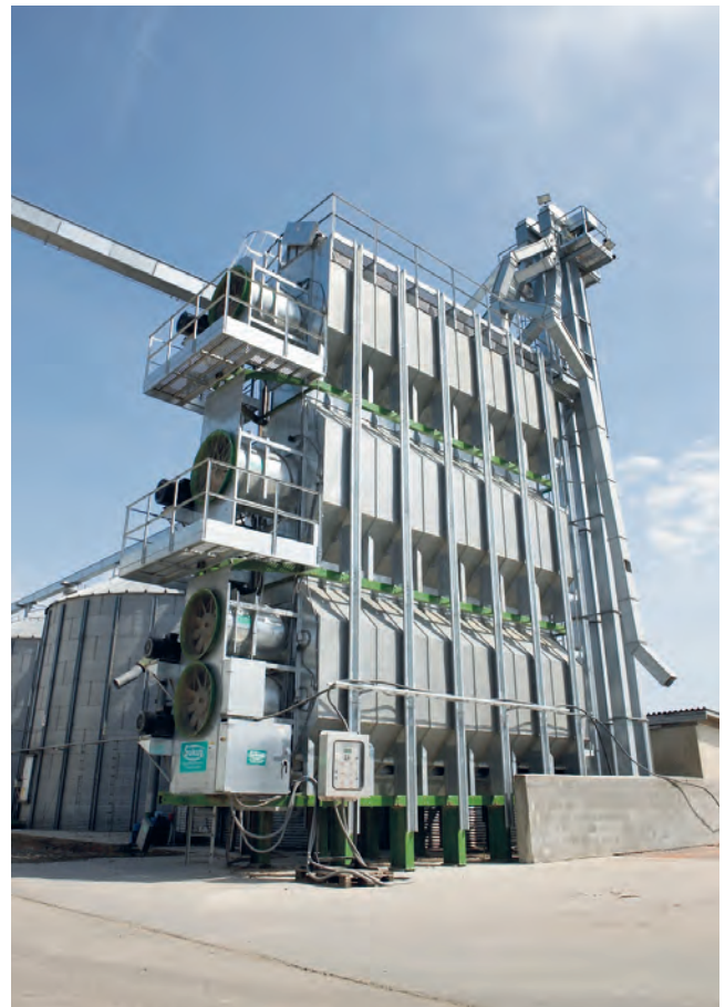
2 module stack dryers with capacities up to 78 t/h 3 module stack dryers with capacities up to 117 t/h
