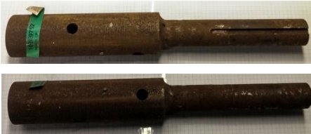
E9752 – Shaft, 10", vertical, bottom, for 1 ¼" bearing.
