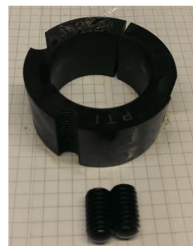
204101610038 - Taperlock For vertical Ø38 5,5 and 7,5 Kw. motor
