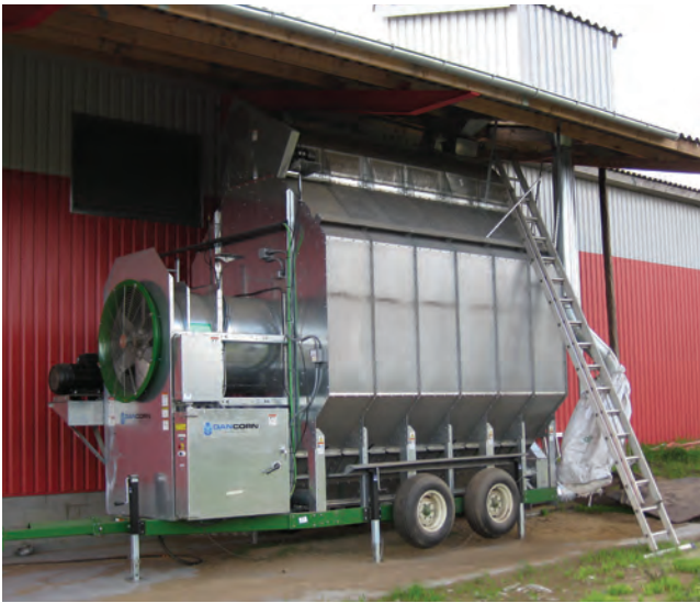
▲ DC 12 mobile dryer with axial fan
